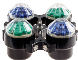
Z446-750 Swing out rotor with round buckets
